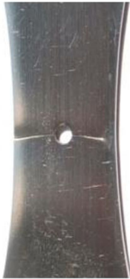
Fig. 14 A portion of the specimen showing the path of crack propagation
